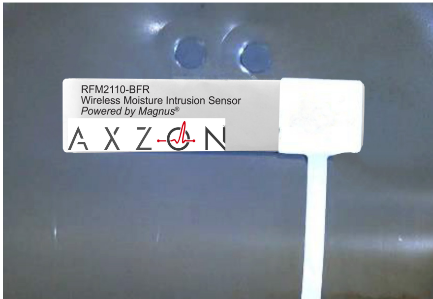
Figure 4: Thin wireless moisture intrusion sensor installed on bare chassis metal with an optional wicking tail that extends the monitoring zone.
